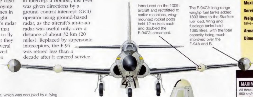
The earlier-production F-94B bore a stronger resemblance to the TF-80C (later redesignated T-33) from which it was developed. The F-94C introduced a swept tailplane, a broader rear fuselage and wing-mounted rocket pods.
